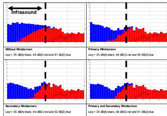
Figure 4: Measurement Results (exemplary); airvelocity: 0,2 m/s (airpressurefield from fan)
